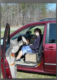
The Glide 'N Go transfer seat single fold version is available for trucks, vans, and SUV's
